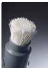
Atlas Copco's innovative Membrane Nitrogen Generator uses membrane air separation to produce nitrogen. The membrane consists of a bundle of hollow fibers with a polymeric structure. The membrane allows nitrogen to pass and other gases (such as oxygen, water vapor and CO<sub>2</sub>) to permeate. Compressed air enters at the inlet of the generator, and nitrogen exits at the outlet. Membrane technology generates nitrogen with a purity between 95 and 99.5% and flows up to 209.9 m<sup>3</sup>/h.
