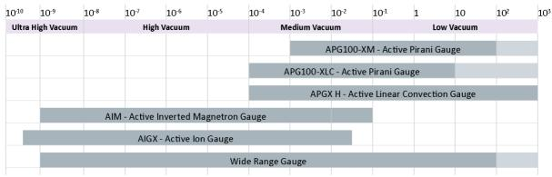
The dark grey shading indicates the primary accuracy range for the specified gauge.
